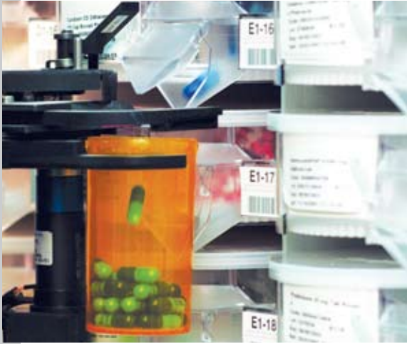
Robotic arm counts and fills without cross-contamination.
