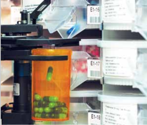
Robotic arm counts and fills without cross-contamination.
