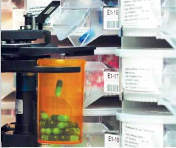
Robotic arm counts and fills without cross-contamination.
