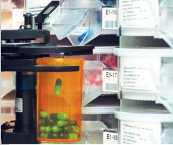
Robotic arm counts and fills without cross-contamination.
