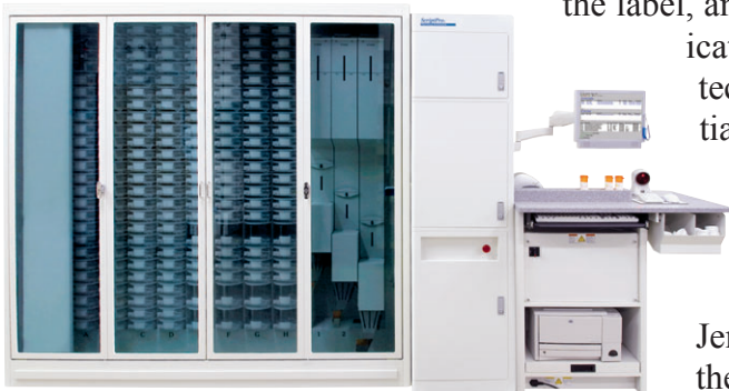
ScriptPro's SP 200® dispenses medication directly from the cell into a vial therefore avoiding cross-contamination.
