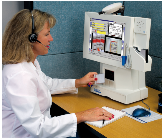
At the central, or support pharmacy, a pharmacist verifies the prescription by viewing on screen the original written prescription, the patient's information, the filled vial, and the drug image before transmitting approval.
