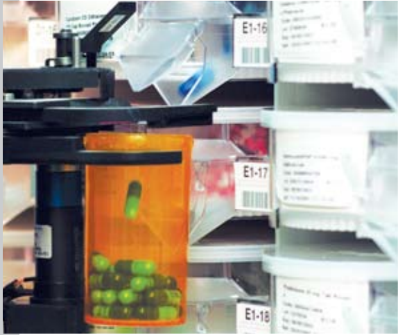
Robotic arm counts and fills without cross-contamination.
