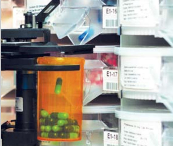
Robotic arm counts and fills without cross-contamination.
