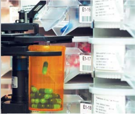
Robotic arm counts and fills without cross-contamination.
