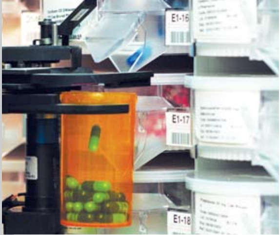
Robotic arm counts and fills without cross-contamination.
