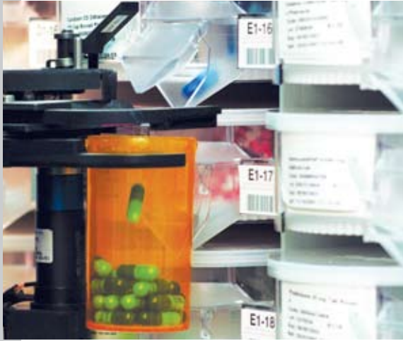
Robotic arm counts and fills without cross-contamination.
