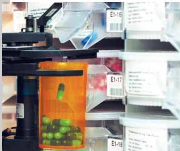
Robotic arm counts and fills without cross-contamination.
