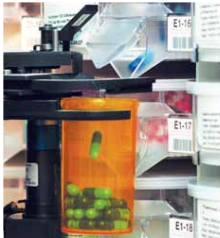
Robotic arm counts and fills without cross-contamination.
