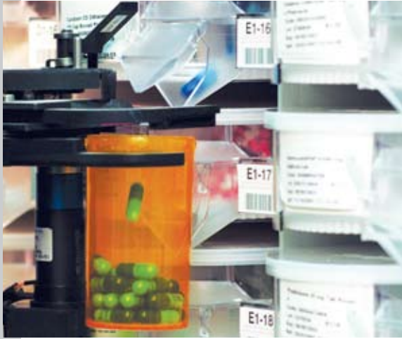
Robotic arm counts and fills without cross-contamination.
